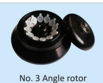
Max. Speed: 13000rpm Capacity: 12 x 5ml Max. RCF: 12750xg ØxL: 14x51mm
